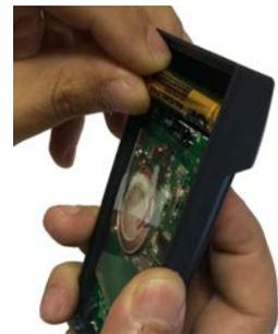
Figure 5 - Insert Battery
