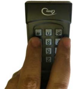
Figure 4 - Reset Keypad to Default Settings
