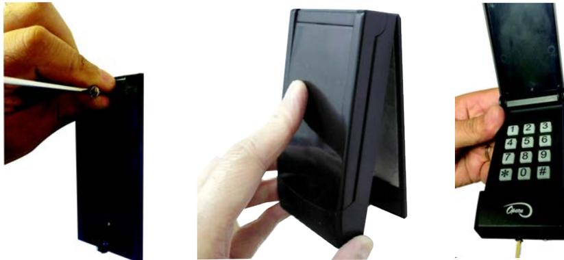
Figure 3 - Mounting KEYLESS042
