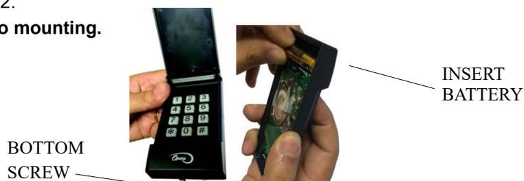
Figure 2 - KEYLESS042 Battery Installation
