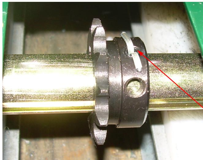
The legs of **PIN 002** are bent around the hub of the sprocket securing the components together
